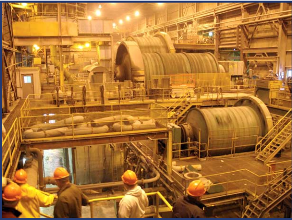
Figure 42a. Large cylindrical mills grind the ore from football size blocks to silt.
