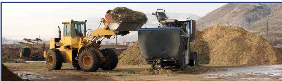
Figure 58. Green waste is loaded into a grinder at the compost facility. Grinding is essential to the composting process as it increases the surface area that bacteria can colonize and digest. (Photo by R..Turner)
