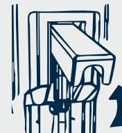
Open the station's door and pull out the connector.
