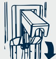
Open the charge port by pushing on the left side of the cover, and then remove the plug cover. Replace it in its socket and close the door.
