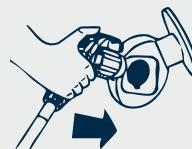
The charge port is on the passenger side. Open it by pushing on the left side of the cover and then remove the plug cover.
