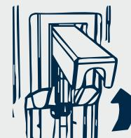
Open the station's door and pull out the connector.
