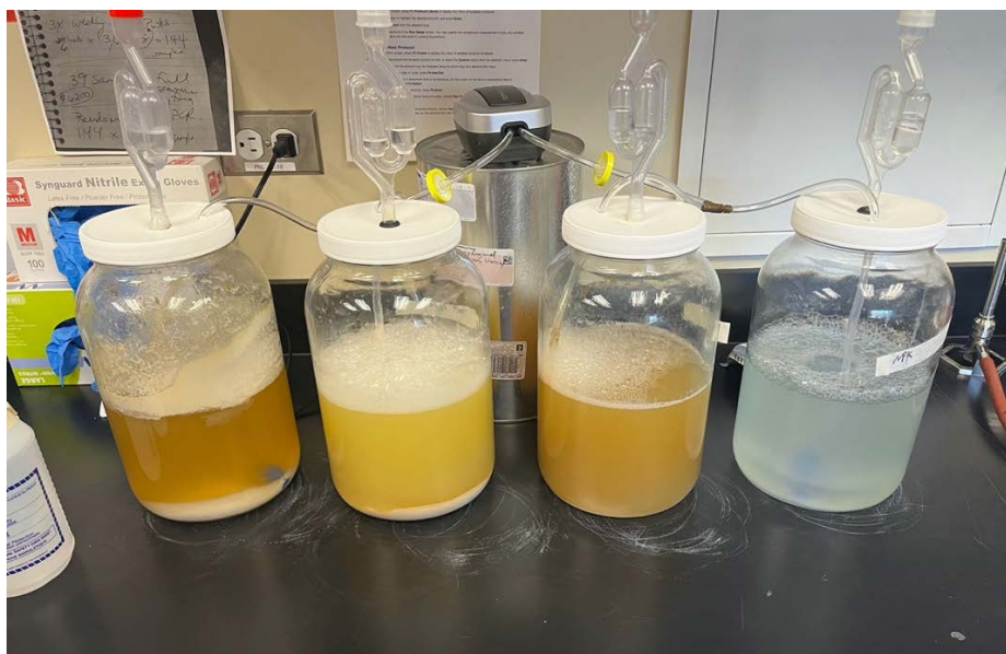
Figure 2.3: Bioreactor setup designed to replicate field conditions, showing air stones (blue), airlines routed through the lids, upstream syringe filter (yellow) behind the central bioreactors, airlocks integrated into the lid centers, and the central air pump.
