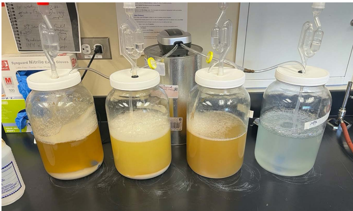
Figure 3.1: Bioreactor setup designed to replicate field conditions, showing air stones (blue), airlines routed through the lids, upstream syringe filter (yellow) behind the central bioreactors, airlocks integrated into the lid centers, and the central air pump.
