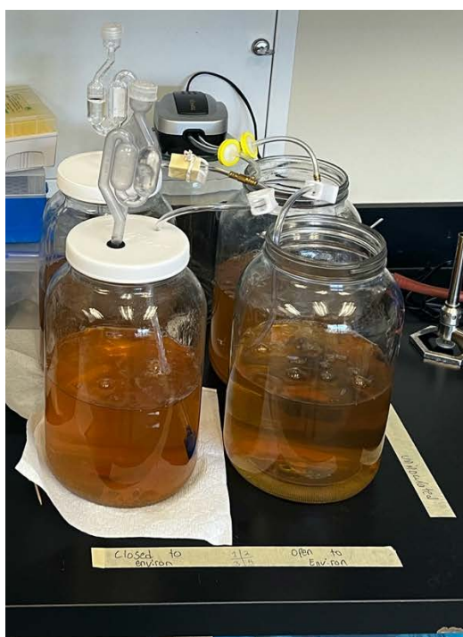
Figure 4.7: Bioreactor and airline set-up for the evaluation of the effect of bioreactors being open to the surrounding air, note only 2 bioreactors have lids while the other 2 are open to their surrounds
