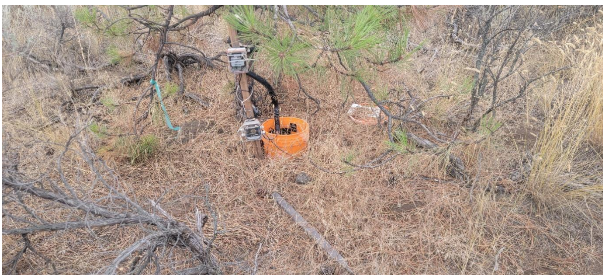
Figure B.2. Tree M-4's stemflow collection apparatus (Sep. 2022).
